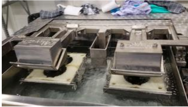
Figure 3.14: Hamburg Wheel-Track Testing Apparatus
