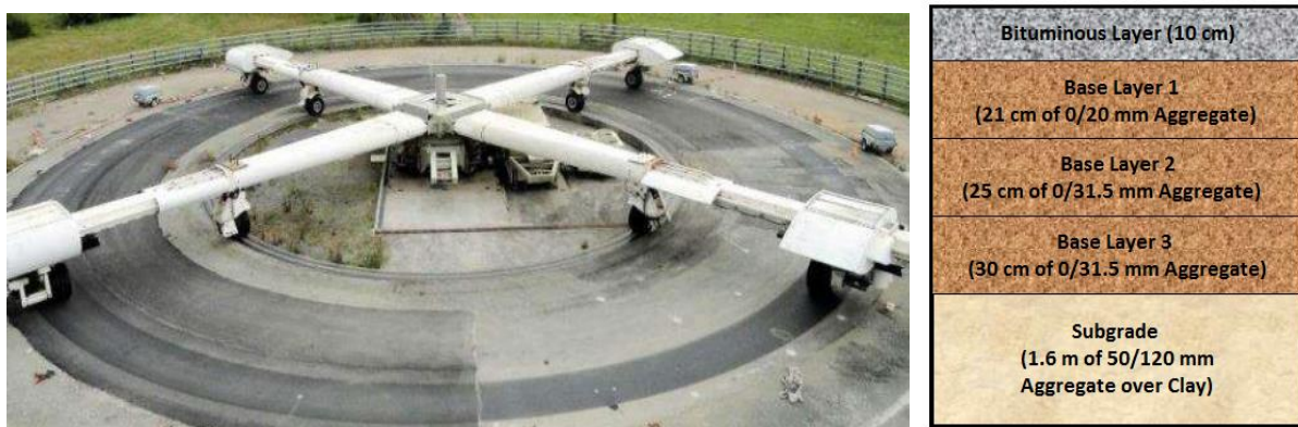
Figure 4.2: IFSTTAR Accelerated Pavement Test Track
